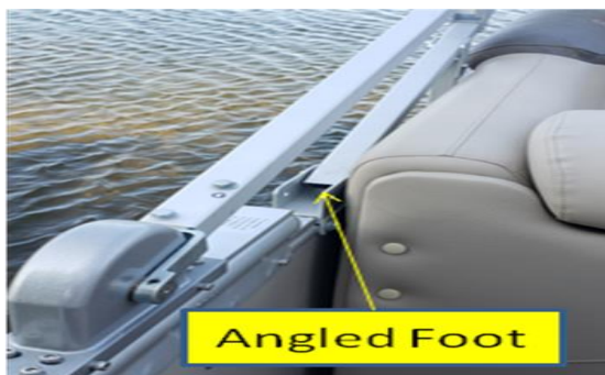
Angled foot on riser attached to rear arch bracket
