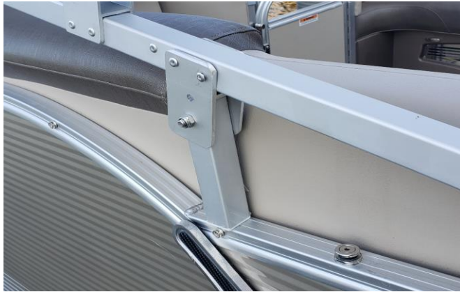
Rear support foot mounted on autobimini aluminum 4 th riser and positioned to avoid interference with boat upholstery.
