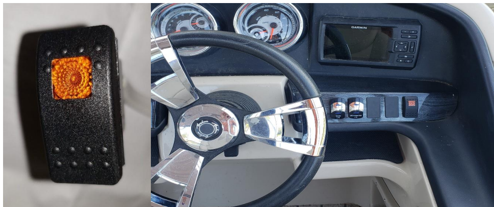
autobimini console switch; console switch installed in helm control panel
