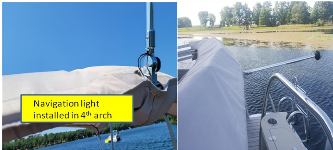
autobimini with navigation light installed in 4 th arch
