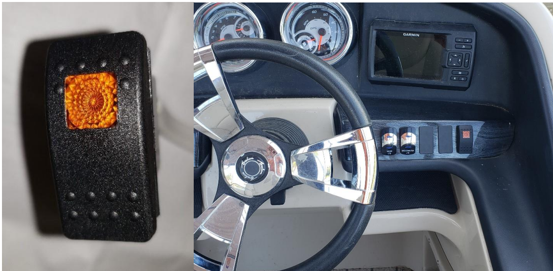
autobimini console switch (left) and console switch installed in helm control panel (right)
