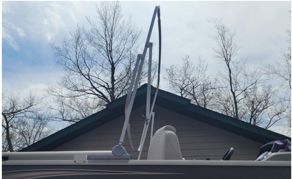
autobimini actuator installed, shown with wire routed through playpen (hidden)
